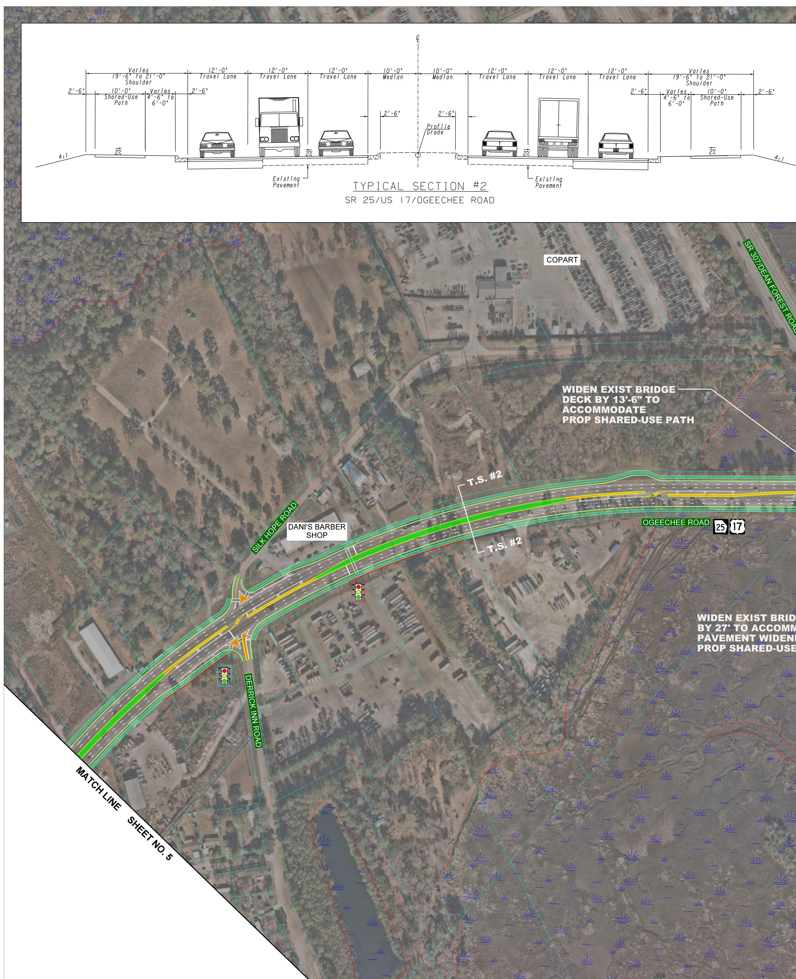
WIDEN EXIST BRIDGE DECK BY 27' TO ACCOMMODATE PAVEMENT WIDENING AND PROP SHARED-USE PATH
